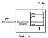
The disc changer consists of a playing unit and a stocker which transports the discs to the disc slot and the playing unit.
